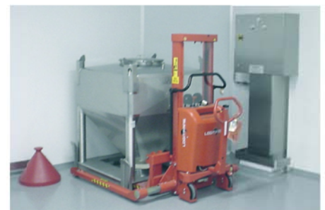
IBC loaded to Discharge Station
