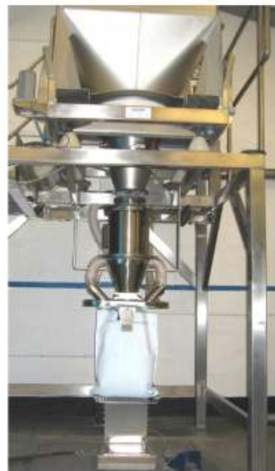
Fig 2: "Direct" packing from IBC through sieve to 25kg bags.
