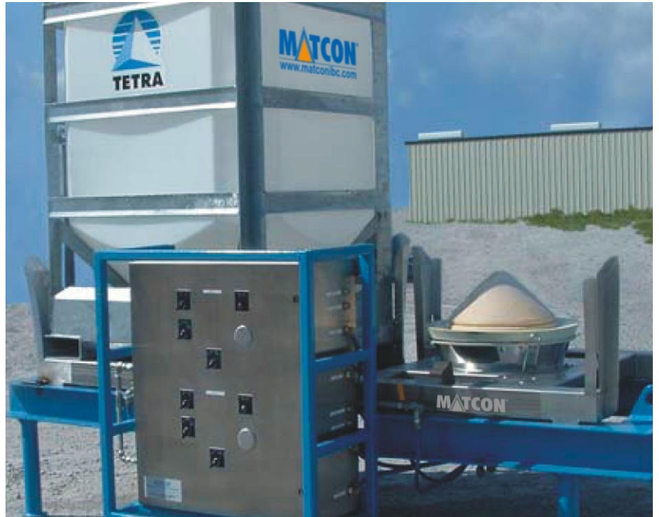
MATCON IBC & CONE VALVE Discharge Station integrated into TETRA's SafeDEflo automated DE delivery system
