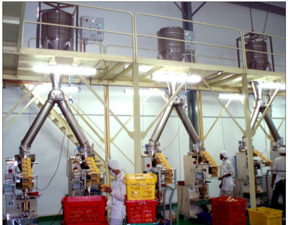
Packing lines fed by Matcon "Smart Drum" IBCs
