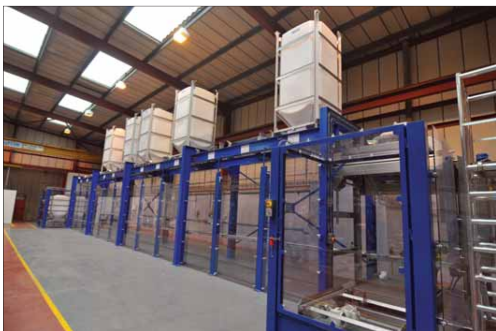
"Flexibatch" automated recipe formulation system undergoing factory acceptance tests before despatch to a customer in Africa.
