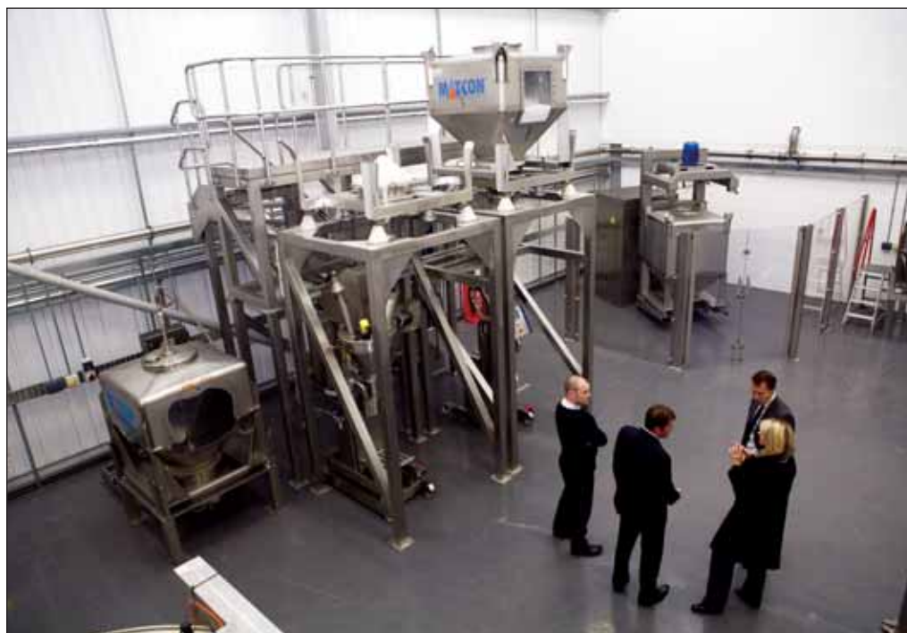
Matcon's in-house test facility in the new headquarters which includes IBC equipment for minor and micro formulation, blending, consumer and B2B packing as well as washing.
